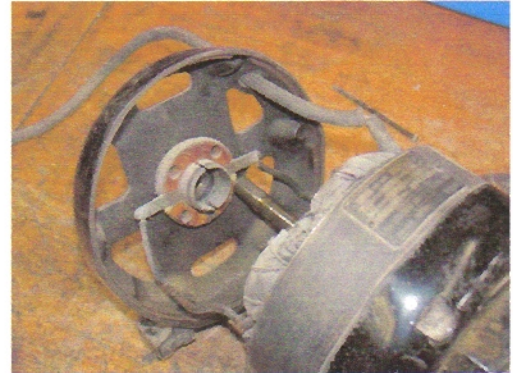
A dirty motor with the front shell removed, shows stationary slip ring pair.
