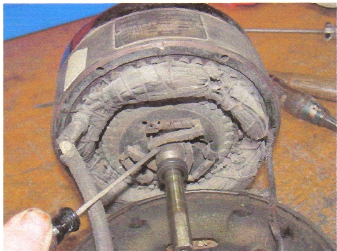
Three spring loaded contacts on the armature of a dirty, unserviced split-field motor. They are beveled and likewise the slip rings, so that they can be spread open and ride the slip rings again when the front shell is replaced.
