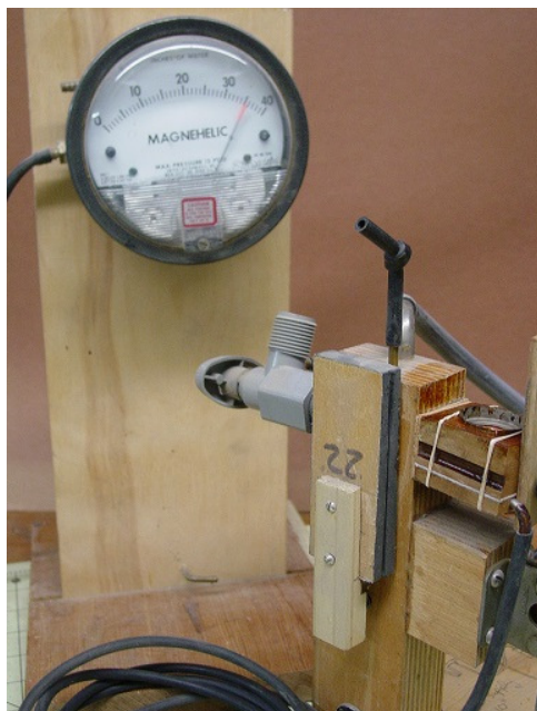
Unsealed White leather pouch actuating on 10.5 ft. of tubing with a tracker bar nipple in one end. As you can see, pouch is not very responsive.
