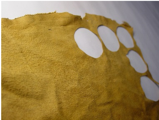
Scruffy and porous, this section of pouch leather has areas which are unsuitable for pouches, but other areas are just fine. You must select your leather in the skin itself.
