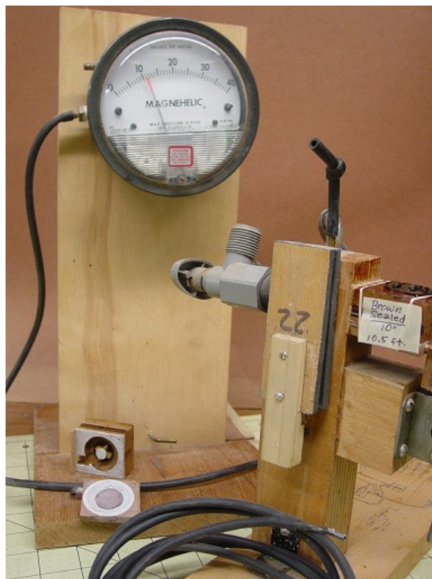
White sealed pouch tested exactly the same as the brown sealed leather and there was no difference at all. Proof that the variable was not suppleness of the brown leather, but the porosity of the white leather.
