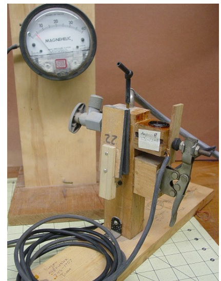
Ampico B valve reference. Operates flawlessly and quickly at 3" on 10.5 ft of tubing.
