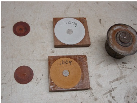
These are the two pouch boards used. Dipping tool on the right. Note ¼" leather spot ready to receive lifter disk.
