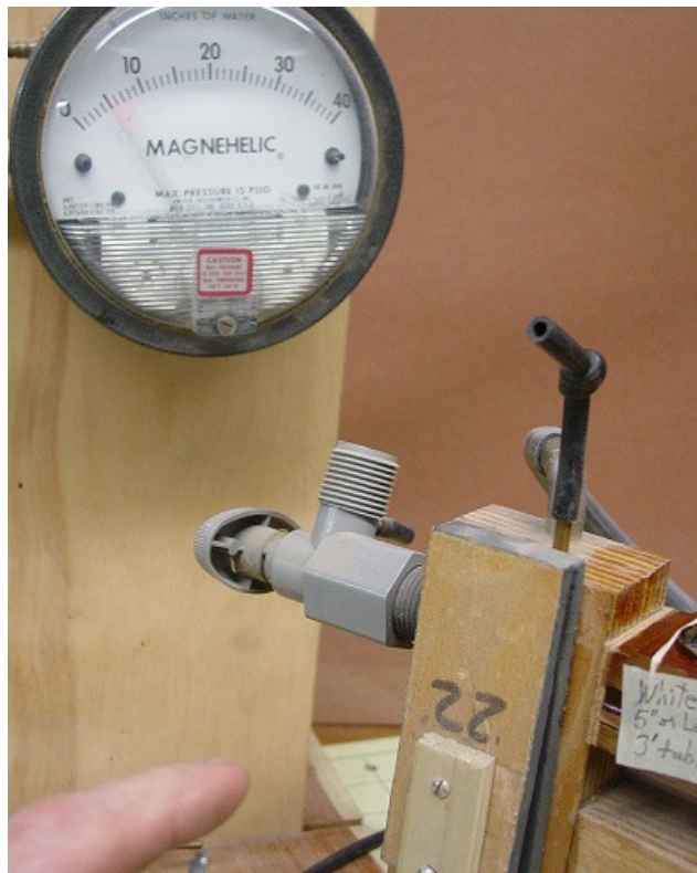
Unsealed White leather pouch operates normally on about 5" vacuum with 3 ft. of TB tubing, but not on any more. Blurry needle caused by finger repetition. Note pneumatic fully closed.
