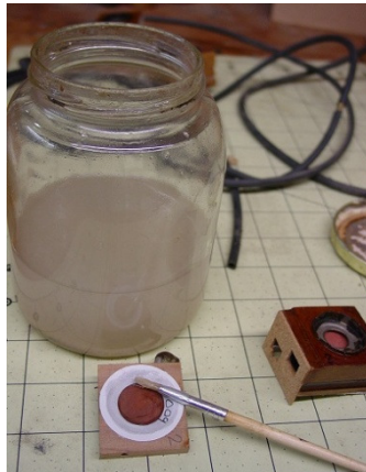
After Pouch has been tested unsealed, it is then sealed to test again. Valve block on the right is leather gasketed on its bottom to seal it to the pouch boards.
