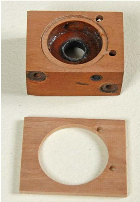
Several pieces of 1/8" thick mahogany were drilled using a 1-3/8" diameter Forestry bit, the same as the Pouch Well, just in case Ron comes across more valves that have to be laminated.
