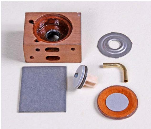
Here are the new parts ready for installation. The shoulder where the Pouch Assembly will be glued has been coated with thin hide glue as a sizing, and the inner surfaces and channels of the block have been coated with shellac to reactivate the old shellac seal. The hide glue sizing provides a good bond for the gluing in the Pouch Assembly as well as keeping shellac from interfering with the glue bond.
