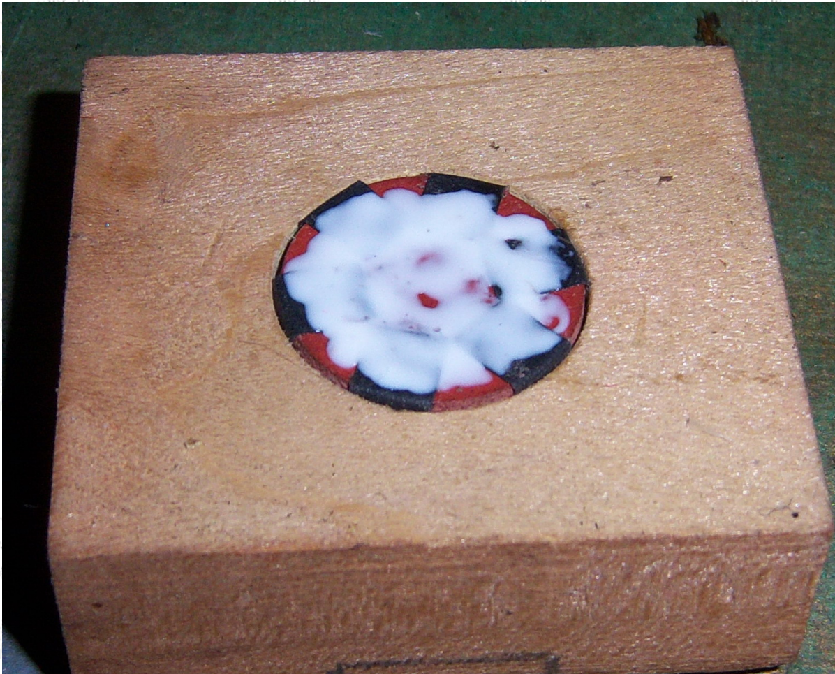
Applying glue for the exhaust facing felt
