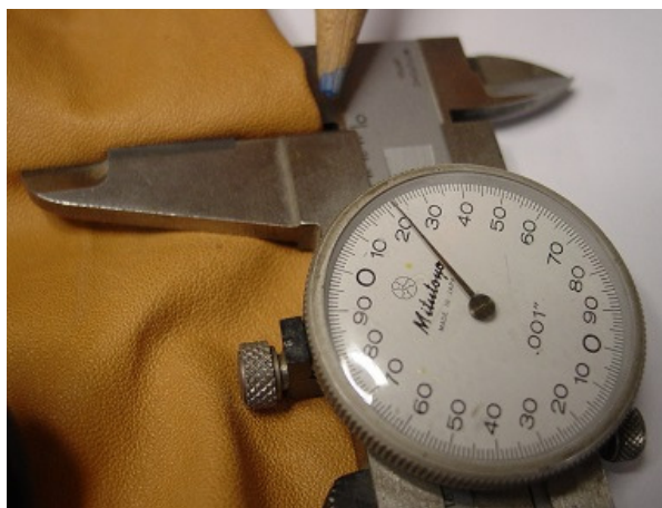
Soft tan pouch leather shown doubled. But the actual pouch cut from this leather was selected from a place where it measured .009" too. Exactly the same as the white leather.
