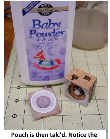
Pouch is then talc'd. Notice the leather gasket under each valve block, allowing each pouch to be tested on each valve.
