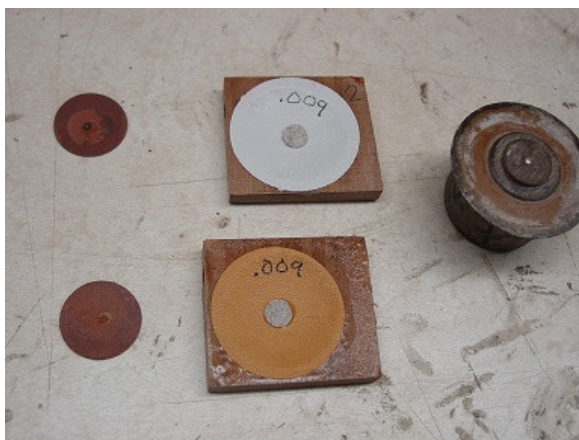
These are the two pouch boards used. Dipping tool on the right. Note 3/4" leather spot ready to receive lifter disk.
