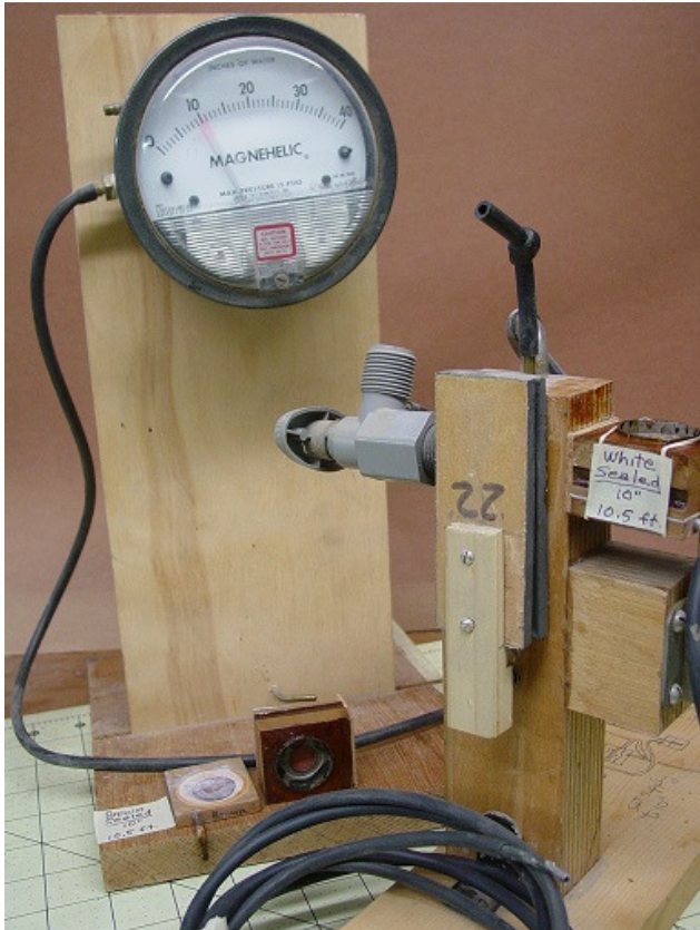
Tan sealed pouch tested 10" H 2 O on 10.5 ft. test tubing. Previously unsealed, it required 15" H 2 O to operate on this much tubing.
