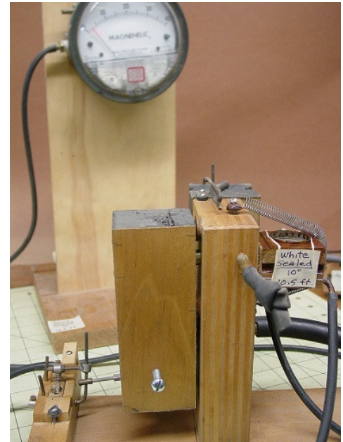
The same white pouch after sealing and its 10.5 ft. sensitivity test is now placed on the rep tester and performs but not as well as the tan pouch.
