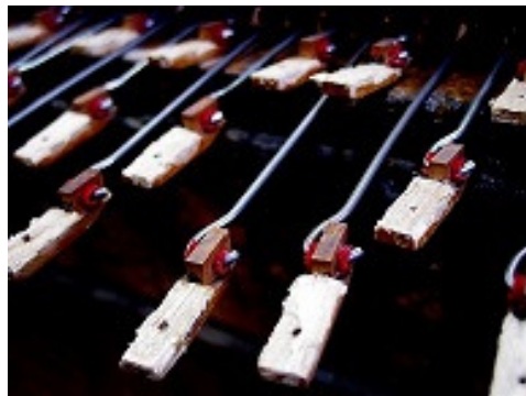
Striking fingers covered with Elmer’s and torn pneumatic wood, forcing removal and individually filing flat to re-glue to new pneumatics.
